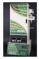
the properties of the sintered materials. The use of non-hazardous supercritical  $CO_2$  in the debinding process eliminates the use of toxic solvents and reduces the time needed to extract organic additives.
