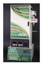
In recent years, alternative techniques for fat determination have been introduced. One of these methods is the extraction of CO<sub>2</sub> under supercritical conditions (SFE).
