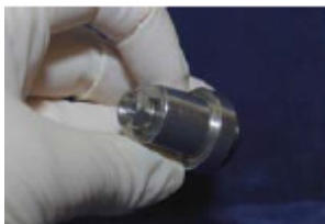
Male fitting goes into endcap.
