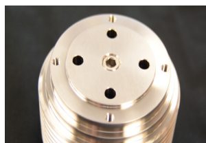
Frit nut screws into cover.
