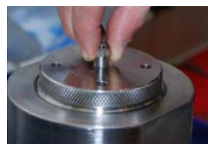
Apply PTFE tape to adaptor fitting 1/8" FNPT to 10-32 THD and attach to cover. (Not necessary to remove every use.)
