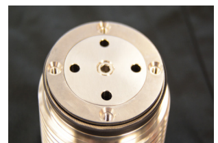
Seal cover fits over seal.
